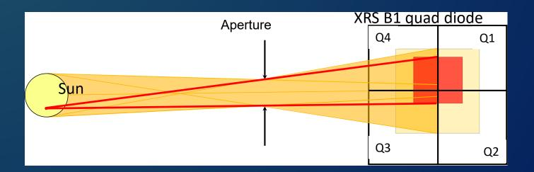
X = [(Q1 + Q2) - (Q3 + Q4)] / QsumY = [(Q1 + Q4) - (Q2 + Q3)] / Qsum where Q1 to Q4 are background-subtracted corrected currents and Qsum = Q1 + Q2 + Q3 + Q4
