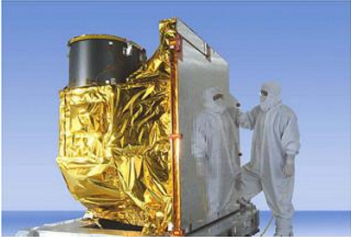
Figure 1: Photo of the Advanced Baseline Imager (ABI). Courtesy of Exelis (now Harris).
