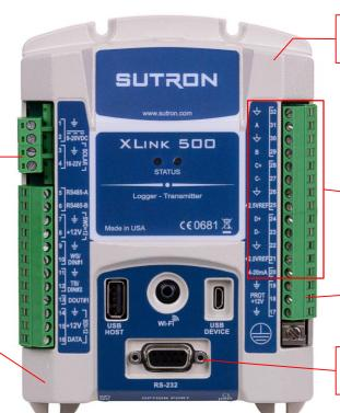
**Lightning protection,** from direct or indirect hits, on all pins.
